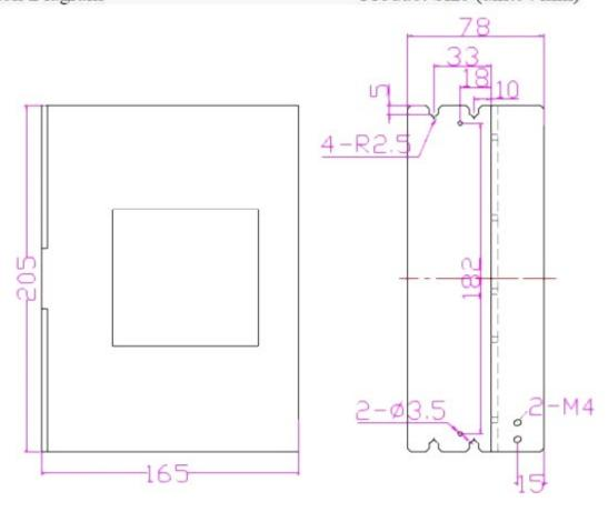
Note: When installing, ensure the equipment well ventilated, and check whether the cooling fan is running normally. When several drivers are used at the same time, ensure the distance between them is not less than 5cm. To ensure safety, be sure to connect the ground protection terminal of the drive to the equipment protection ground.
